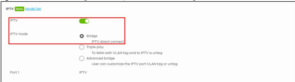
Figure 139 Site-wide > Configure > Security router > Interface: Bridge Mode
